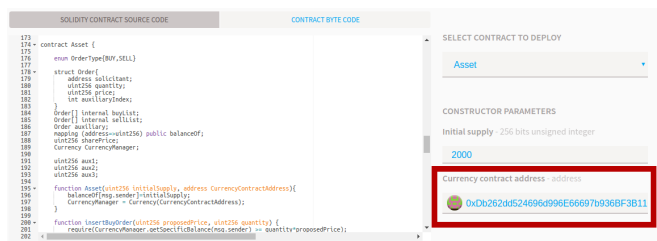
Figure 13. Highlight of the parameters needed to deploy Asset contract.
